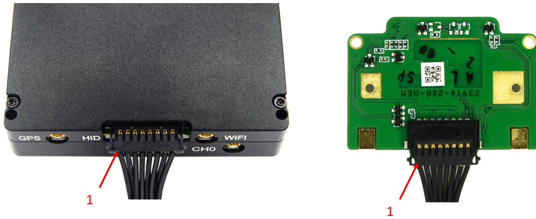
Fig. 2 Connecting the HID Expansion Board to the OEM Radio
